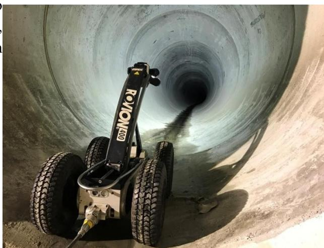
*pipeline CCTV inspection [source: pipevision corporation]*
